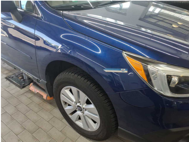
Damage #1: Mudguard - right side: Mudguard - right side - dent(s) - Smooth repair work
