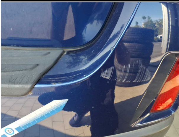
Damage #11: Rear bumper: Rear bumper - Scratch(es) - Repair and paint
