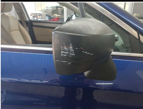
Damage #3: Wing mirror - right side: Wing mirror - Scratched - Replace
