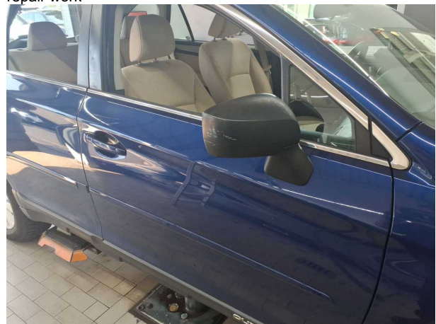
Damage #3: Wing mirror - right side: Wing mirror - Scratched - Replace
