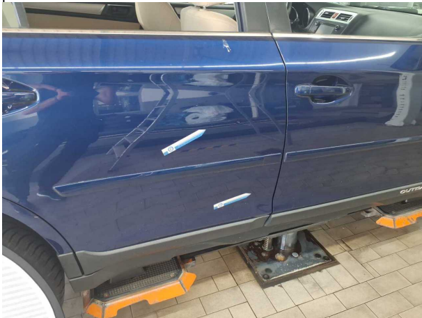
Damage #12: Door - rear right side: Door - Damaged - Repair and paint
